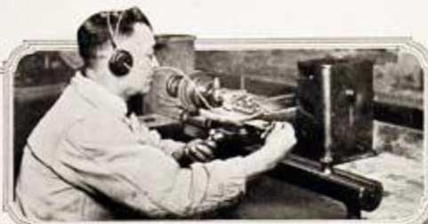
IN THIS INSTRUMENT one diamond is cut into shape by another diamond. The operator listens through his telephone head set and adjusts the diamonds till the right click tells him they are making proper contact.
